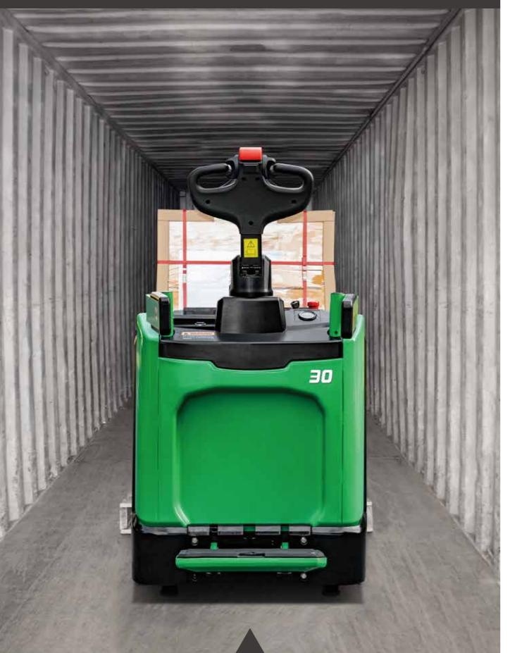
The compact body and large corner design make the truck suitable for work in narrow spaces, and the chassis is designed with a wedge shape, greatly improving passability.
