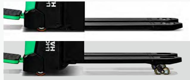
The unique shock absorbing floating suspension system of the stand-on ensures that the driving wheels are always in contact with the ground, ensuring the stability of the truck.
